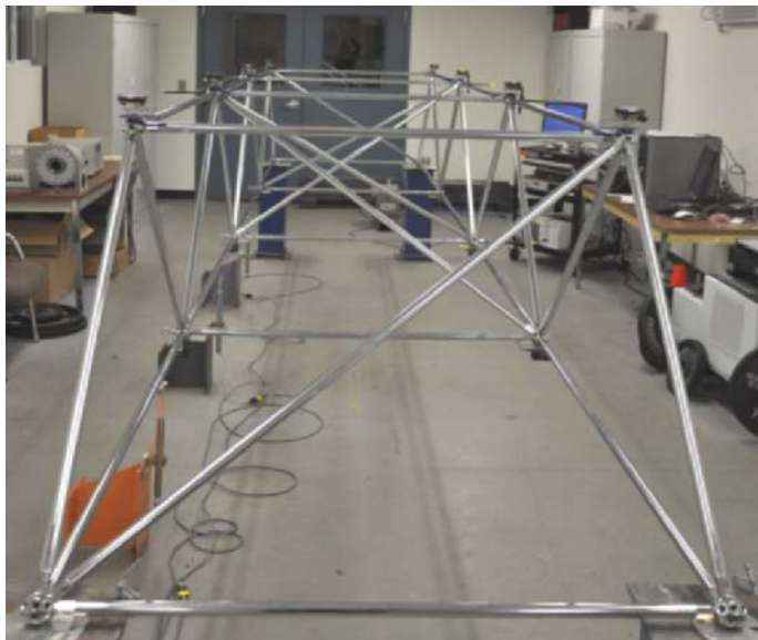
Figure 2, 3-D steel truss of the experiment
