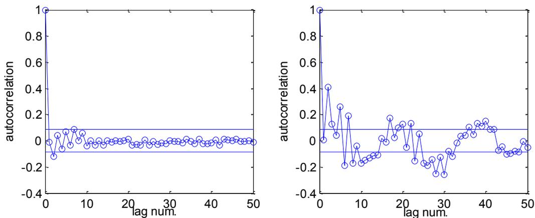
FIG. 2. RESIDUAL AUTOCORRELATION AS DAMAGE INDICATOR; LOTS OF OUTLIERS APPEAR WHEN MODEL NO LONGER FIT THE DATA WELL. THE LENGTH OF RESIDUAL SEQUENCE IS 520.
