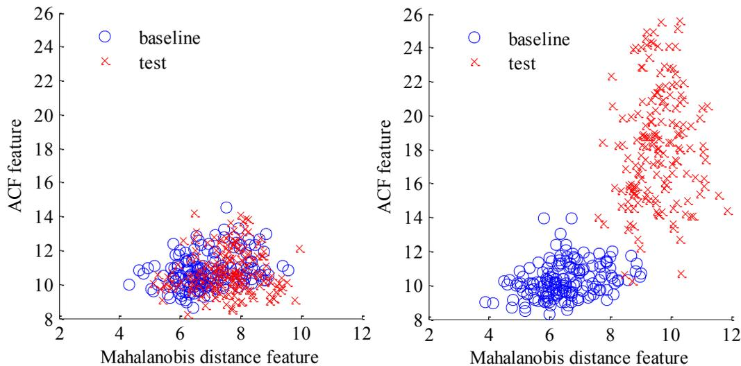
FIG.6 SCATTER PLOTS OF DAMAGE FEATURE PAIRS.
