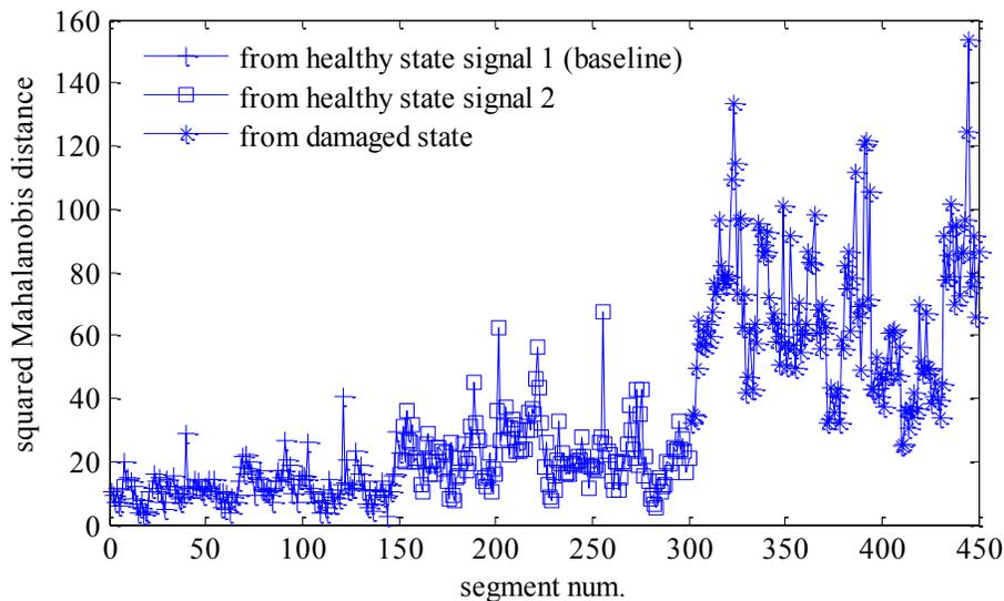
FIG. 1. MAHALANOBIS DISTANCE OF MODEL COEFFICIENTS. SEGMENT SIZE IS 350. THE OVERLAP BETWEEN CONSECUTIVE SEGMENTS IS 300.
