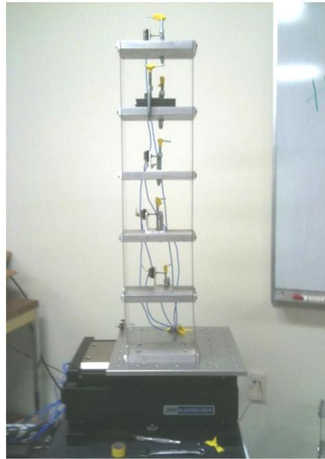
FIG. 4 THE PLEXIGLASS 5 DOF LAB SPECIMEN
