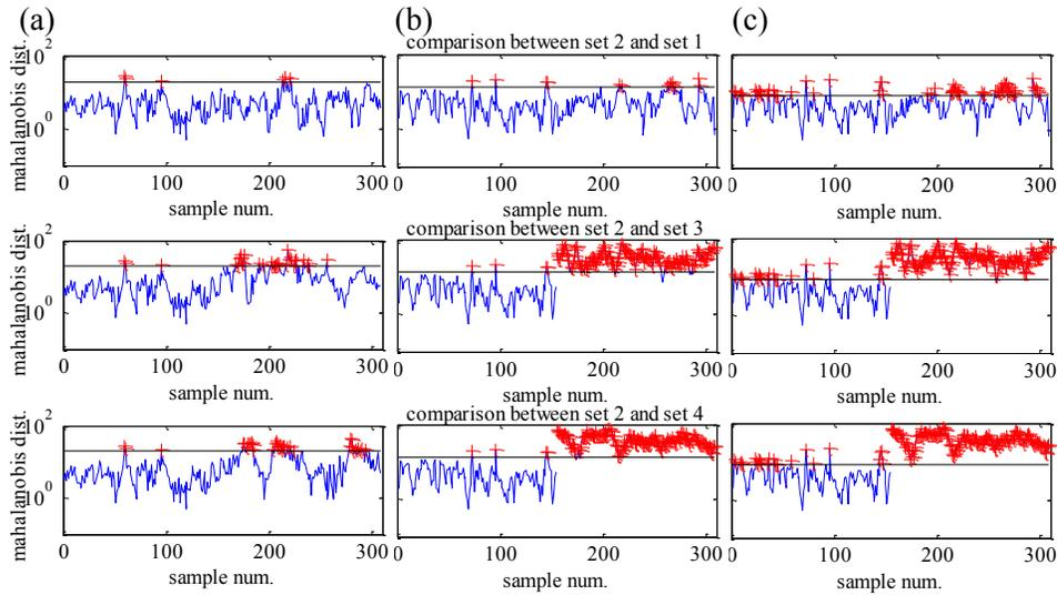
FIG. 5 DAMAGE DETECTION USING THE MAHALANOBIS DISTANCE OF AR MODEL COEFFICIENTS.
